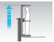
**Shockless Ascent Stop** The system reduces the lifting speed near the end of the ascent stroke, reducing jolting when maximum lift height is reached. Note: Available when the Deluxe Multifunction Display is selected
