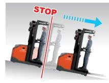
Anti-rollback When the accelerator is released while on a grade, the truck stops and then descends at a constant speed. This helps to ensure operation on slopes.
