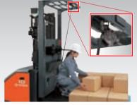
Reel-type Safety Belt OPT The self-retracting extensible belt eliminates slack, enabling the operator to engage in a wide range of operations.
