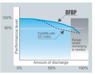
**Power-keep Function** This function boosts load-handling and travel performance as the battery charge drops. This lets you can continue efficient operation. Note: Not available in the H mode.
