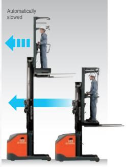
Automatic Vehicle-speed Control This controls vehicle speed as well as acceleration and deceleration according to lift height, achieving both stable travel and good productivity.
