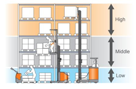
Storage space for infrequently unloaded items and replenishment items at middle- and low-height spaces. Reach trucks are suited to loading and unloading operation.
