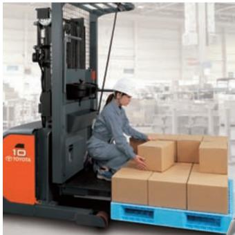
Together with a design emphasis on productivity for order-picking tasks, the low-height battery hood achieves a wide view to the front during travel.
