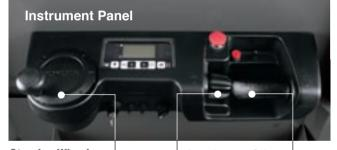
Steering Wheel — The system keeps the angle of the tires corresponding to the angle of the steering wheel. The small-diameter steering wheel also helps reduce operator fatigue.
