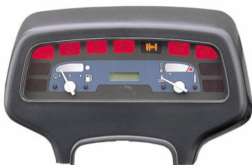
Swing Lock Cylinder indicator light informs operators when SAS is engaged, making them aware of SAS's role in maintaining stability.
